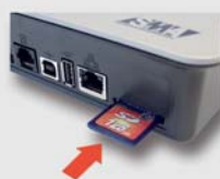
Memory expansion and data transfer to a PC using a removable SD card
